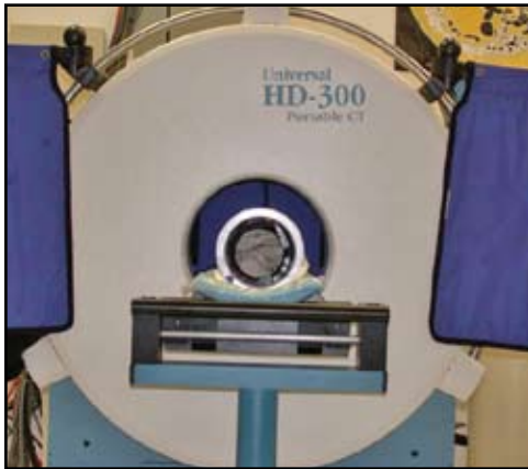
HD-300 system with a 4" core in a AL vessel
